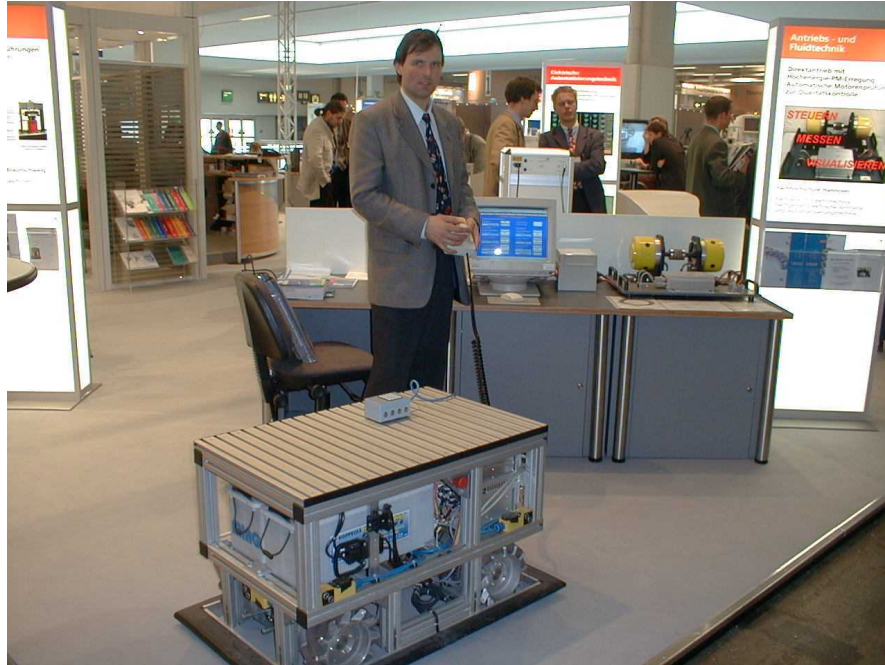
Autonomously guided vehicle system (AGV) for transportation
